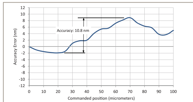
Figure 8. Example accuracy error calculated from the measurement data shown in Figure 7.
