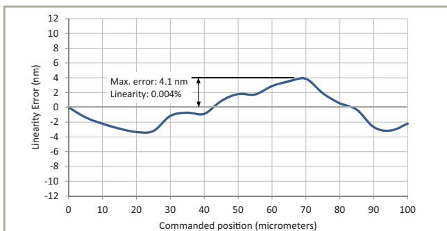
Figure 9. Illustration showing how linearity is calculated based on measurement data taken from a 100 \mu\text{m} piezo nanopositioning stage.
